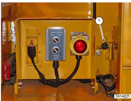
Figure 4. Back-up bleed down valve (ground location access)
